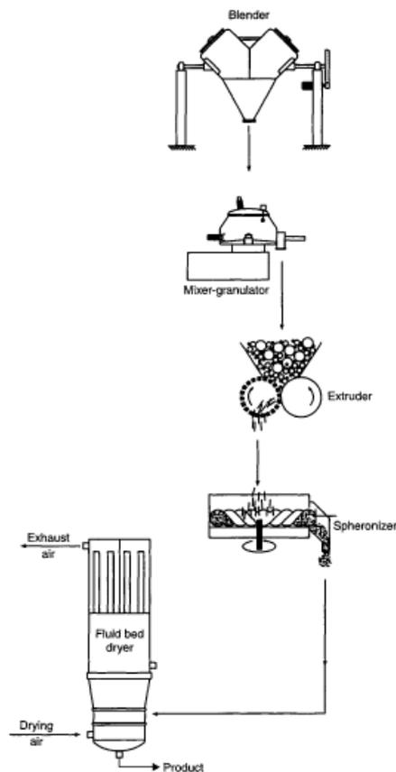
Figure 6.11 Typical spheronization process
