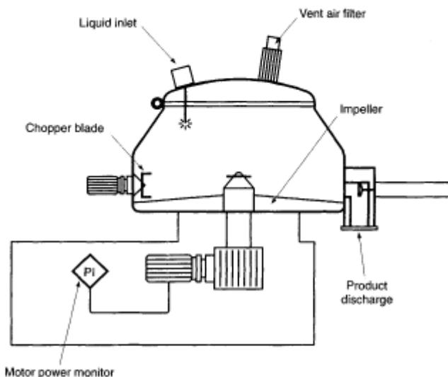
Figure 6.3 High shear mixer-granulator with opening lid
