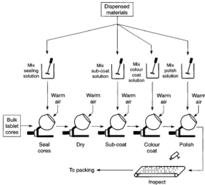
Figure 6.8 Tablet sugar coating
