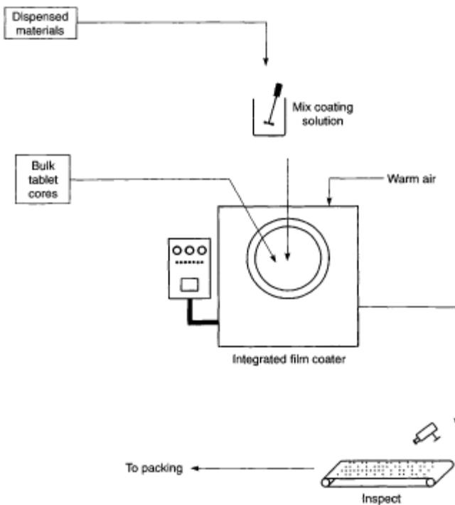
Figure 6.9 Tablet film coating
