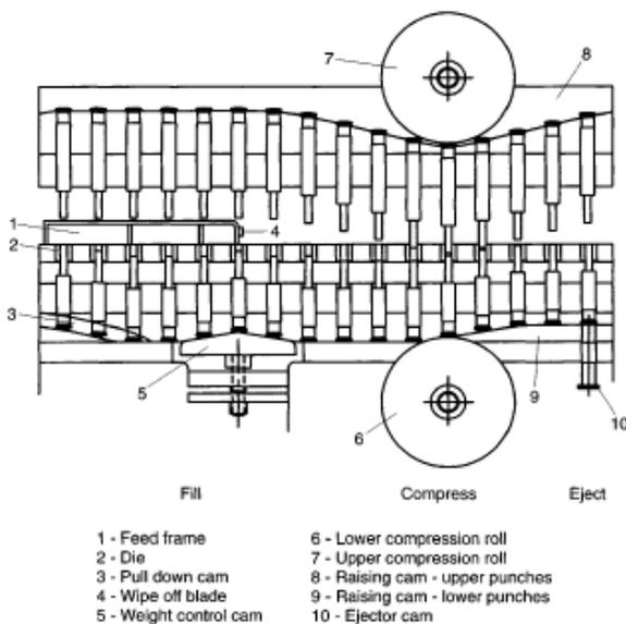
Figure 6.6 Rotary tablet compression machine operation
