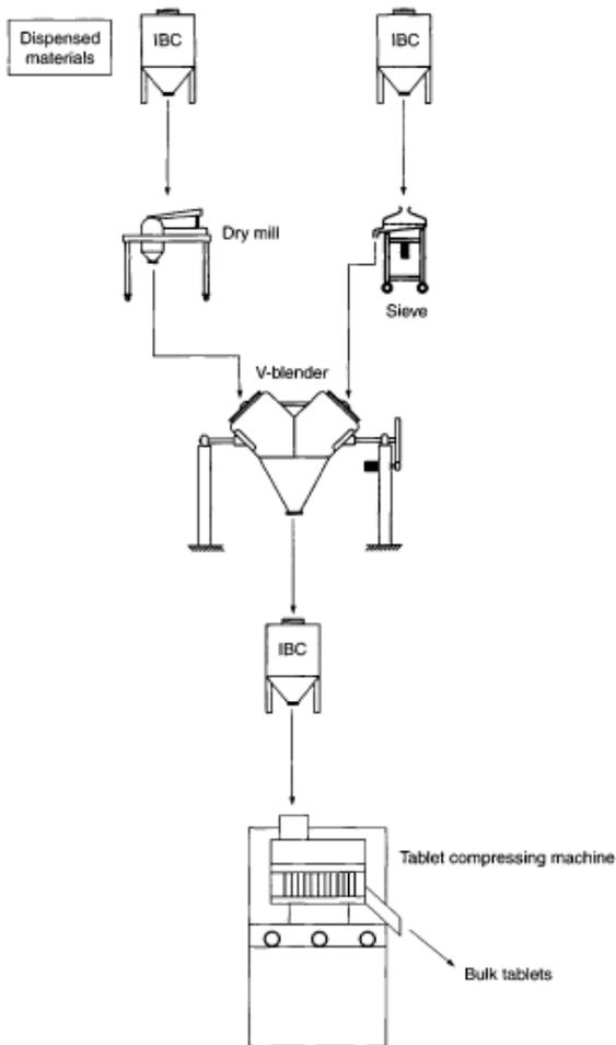
Figure 6.5 Typical flow diagram for direct compression
