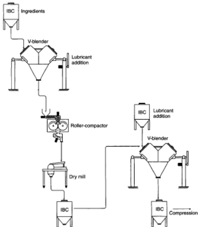
Figure 6.1 Typical dry granulation process
