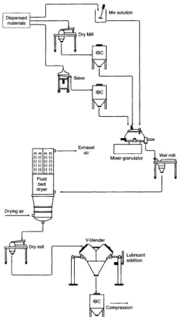
Figure 6.2 Typical wet granulation process
